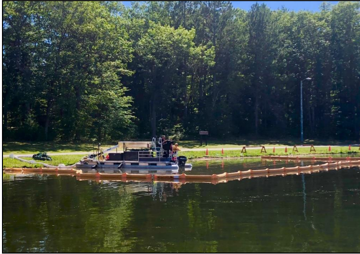
Figure 50. A DASH boat for hand-removal of watermilfoil or other nuisance vegetation. ©Restorative Lake Sciences, LLC
